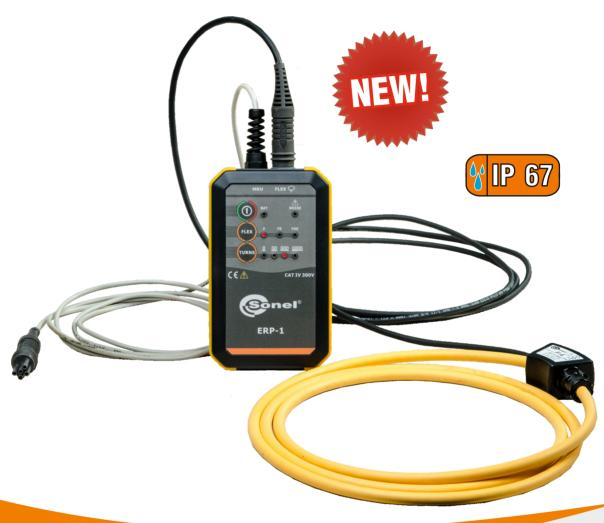
Sonel ERP-1 adapter is used for earth resistance measurements of electricity pylons using flexible clamp - Rogowski coil.
