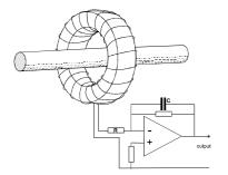
To complete the transducer the coil output voltage is integrated electronically to provide an output which is independent of frequency. By varying the integration parameters (C and R) the sensitivity of the complete measuring system can be varied over about five orders of magnitude. In the DIN1 unit the output of the integrator is converted to a true RMS value which is then converted to a 4 - 20mA DC output.
