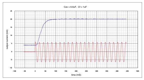
Red trace = current waveform, blue trace = transducer response
