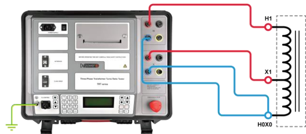
Connecting TRT to a single-phase autotransformer
