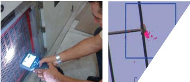
Slim daylight UV testing corona cameras suitable for nearby and remote, in & outdoors operations. Camera stands out for its bright & large LCD, pleasant user interface and elegant and ergonomic design providing an outstanding user experience. Available models SC, VC, SX, VX models. X series has upgraded LCD
