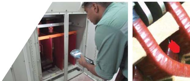
A compact handheld UV testing equipment for illuminated indoors. Point-and-shoot with built in recorder for convenient and safe testing in regularly lit workshops. Efficient in revealing and pinpointing PD in rotating machines and any indoors Hi/Med voltage installations
