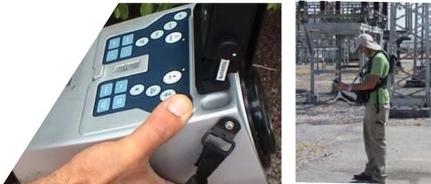
Daylight corona imaging & recording camera with sensitivity features that ensure excellent performance. A robust casing provides for testing within high magnetic & electrical fields. Superb offers reliable precise data and is often mentioned in scientific studies. Uniquely operated through a keyboard. Available models OD | XD
