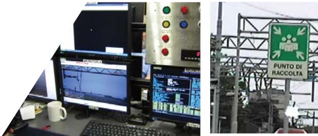
A proprietary automatic corona & arcing monitoring system for overhead railways electrical lines. DayCor® Rail system consists of a high-end detector with a HD recorder, a Corona-Catch processor and a control & display unit. Corona-Catch distinguishes between UV noise and corona, referring only to corona events, thereby streamlining post analysis. Pinpointed corona directs maintenance to suspected faults, reducing inspection workload and making it easier to perform.
