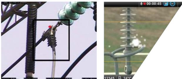
HD corona camera with features that boost corona detection and visualization. LuminarHD is the optimal choice when asking to streamline monitoring tasks. Outstanding optics and sensitivity to UV ensure unparalleled performance and clear display of pinpointed corona from far away and nearby. High definition recording lets users see more when analyzing the recorded media.
